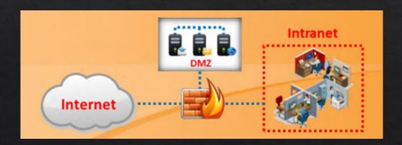
The main advantage with the screened subnet is it separates the DMZ and Internet from the intranet so that when the firewall is compromised access to the intranet won't be possible.
