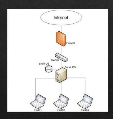
Snort in inline mode creates a transparent bridge between two network segments
