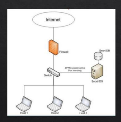
You must mirror the traffic of a switch port or VLAN. For this, we will use the "port mirroring" mechanism which means the switch duplicates the traffic on your chosen interface or VLAN and send it to Snort. On Cisco Catalyst, this is a "SPAN" port You can SPAN one port to another, a group of ports to one port, or an entire VLAN to a port
